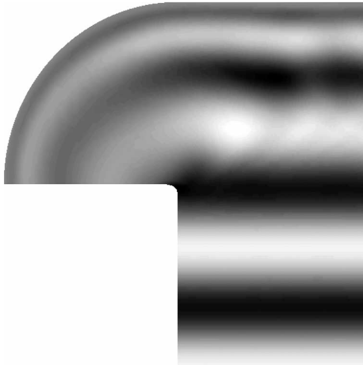
Fig. 10. Wave surface calculated by the present model without wave–current interaction.
